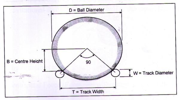
In the above diagram the Ball Diameter is 114mm and the track is 8mm. This gives us an equilateral triangle with the sides equal to the sum of the radius of both the ball and the track. Since we know that the sides of an equilateral triangle are in the ratio of 1 to  $\sqrt{2}$
