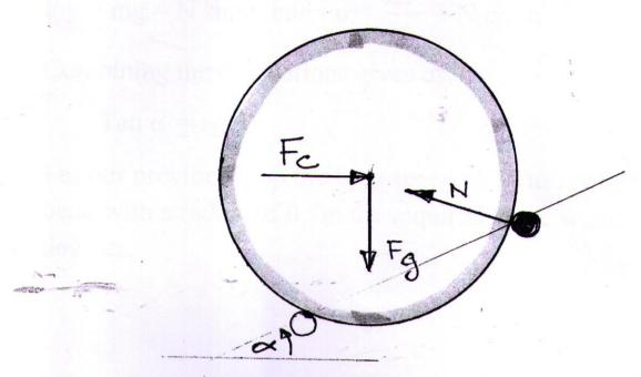
Look at the forces on the ball when it is about to tip off the track. All the weight of the ball will be on the outside track. The normal force off the track will be balanced by a gravitational force holding the ball down with a centrifugal force trying to tip the ball up over the outside track.
