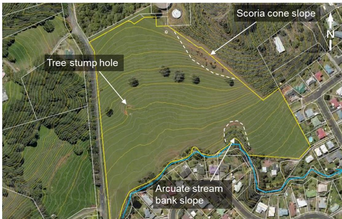
Figure 4: Topographic plan of the subject site with notable site features identified. Contours shown at 1m interval with 5m major contours, falling from north to south through the site. See attached investigation for full scale plan.
