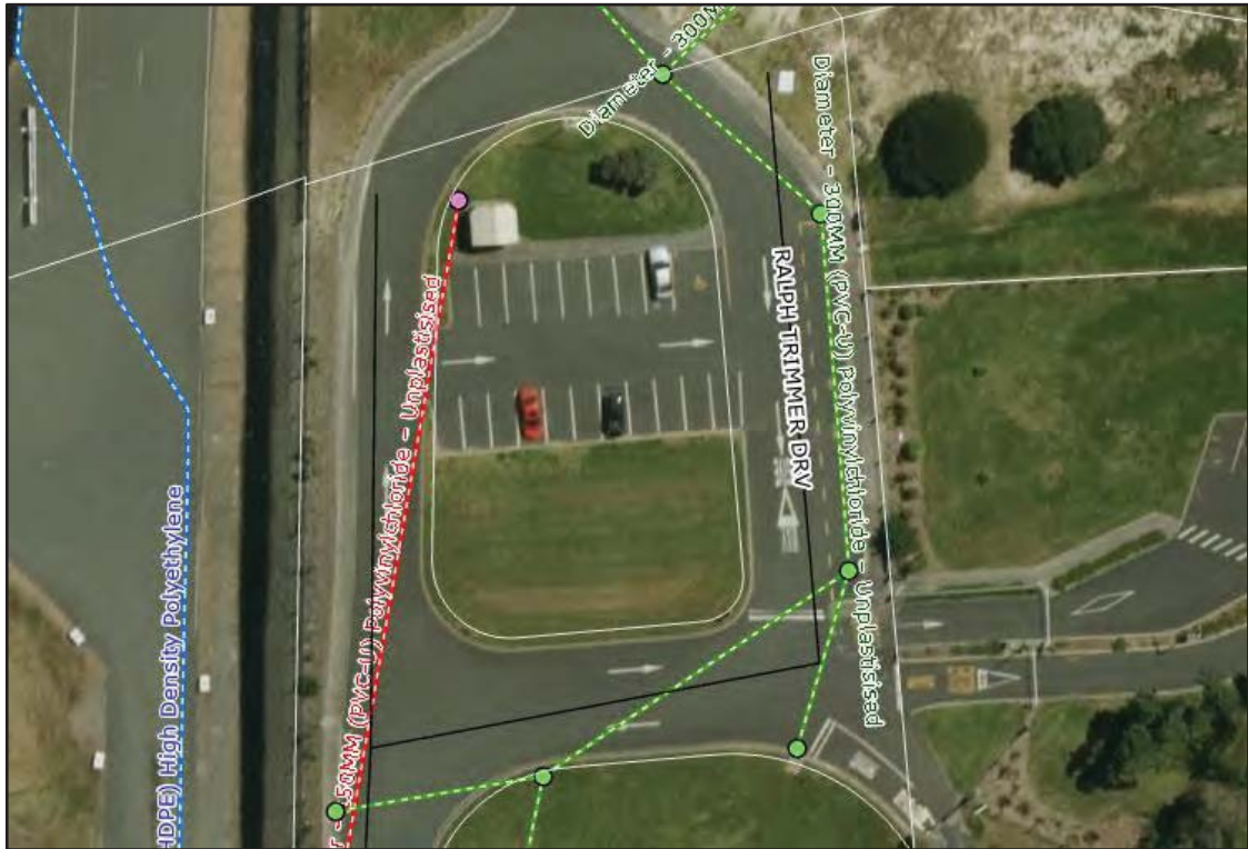
Figure 1: WDC wastewater reticulation (Source: WDC GIS)
