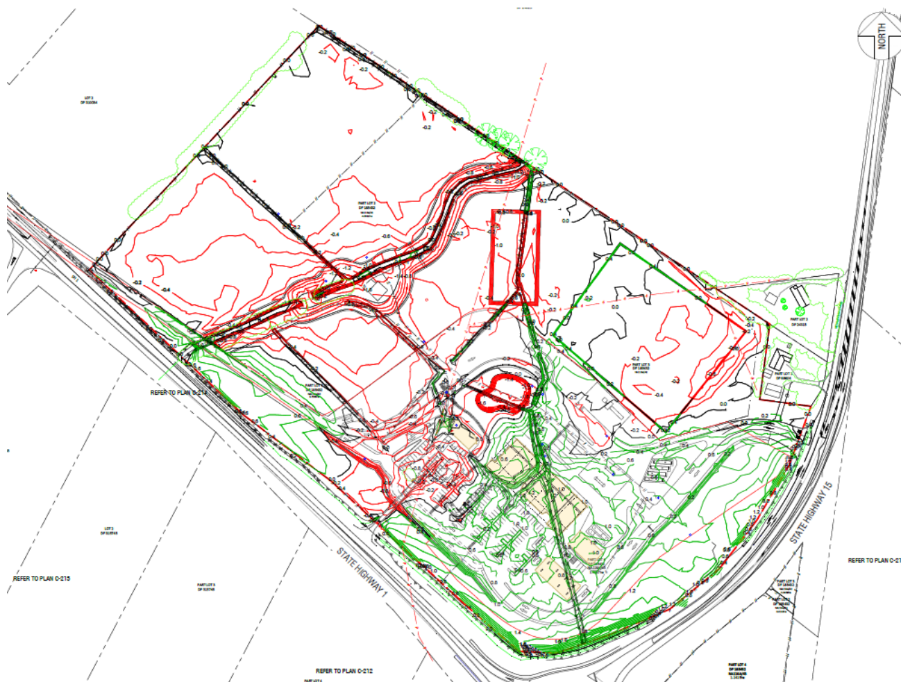
Figure 11: Proposed Earthworks Isopatch plan by Bluebarn Consultants.
