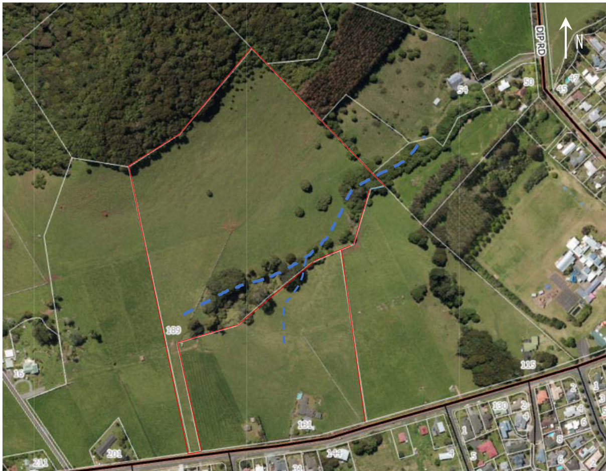
Figure 3 - Aerial photo of sites (red) with the adjacent flow paths indicated in blue. Sourced WDC GIS.
