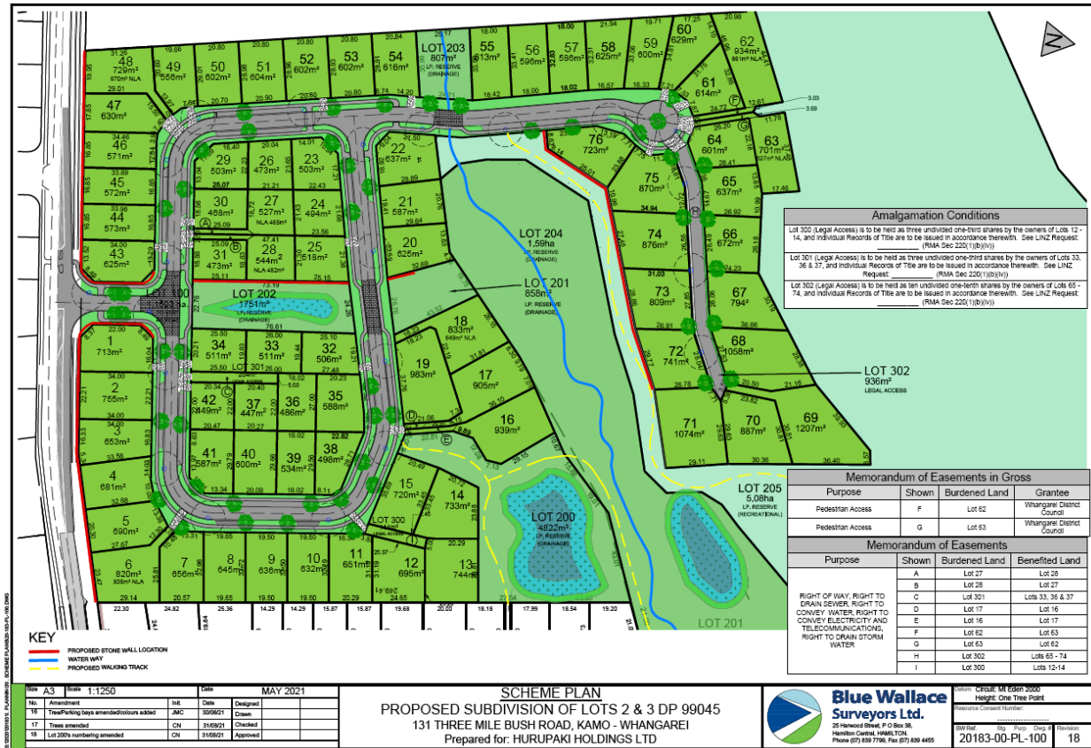
Figure 3: Scheme Plan for the proposed subdivision at 131 and 189 Three Mile Bush Road, Kamo (Blue Wallace Surveyors - May 2021)
