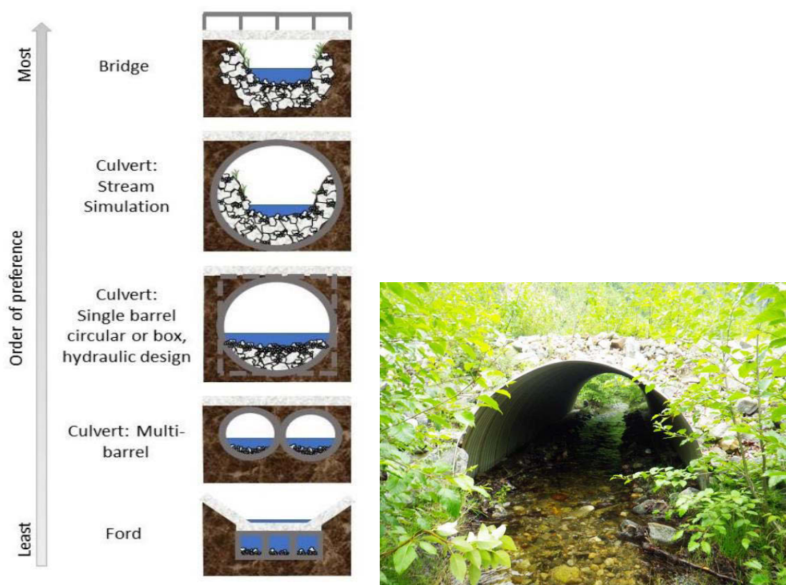
Figure 28: Order of preference for road crossing design, based on the degree of connectivity (left), and (right) showing an example of a stream simulation culvert design (most preferable option)
