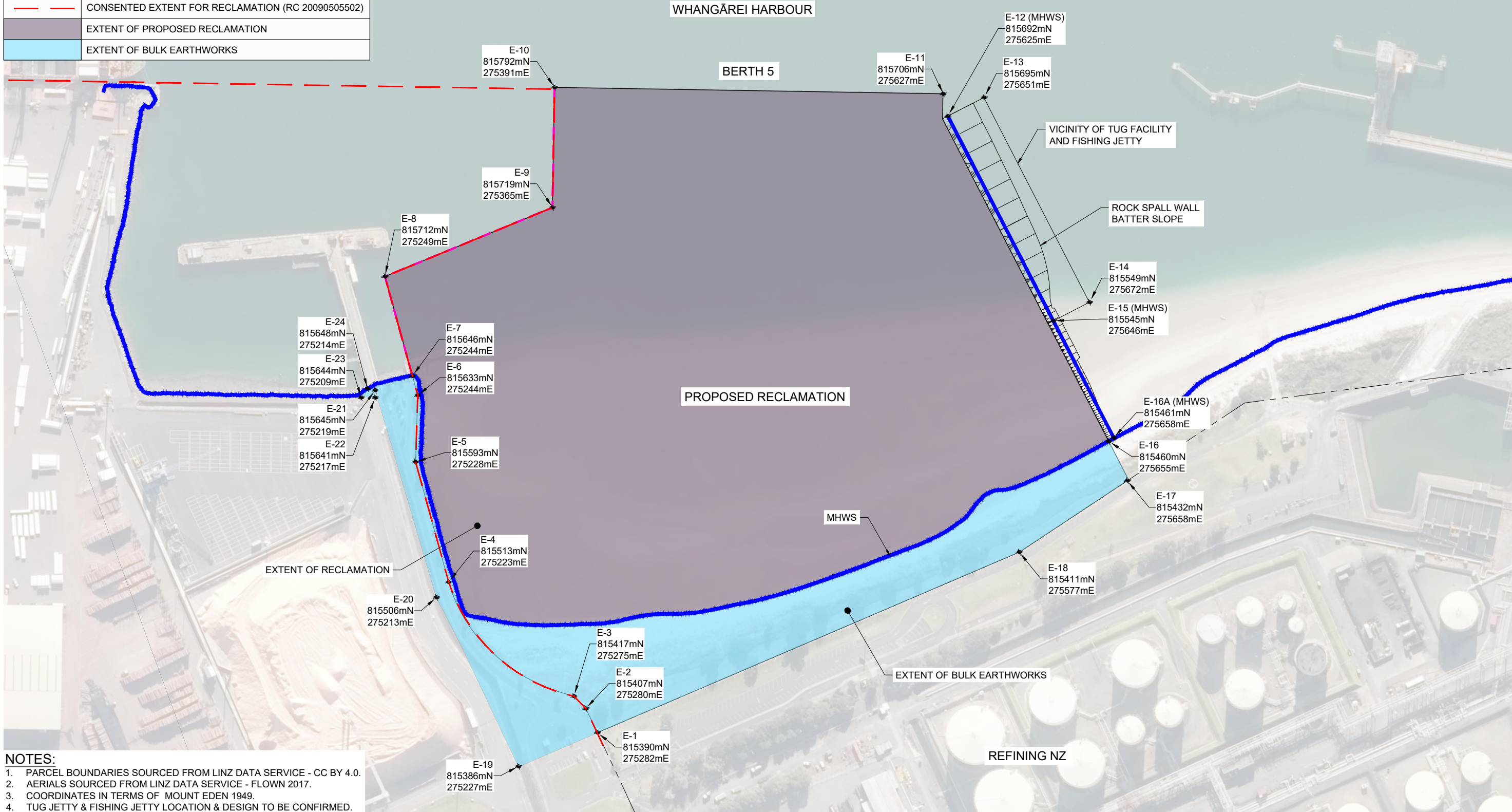
SETOUT PLAN - EASTERN RECLAMATION AND WHARF EXTENTS SCALE 1:1250
