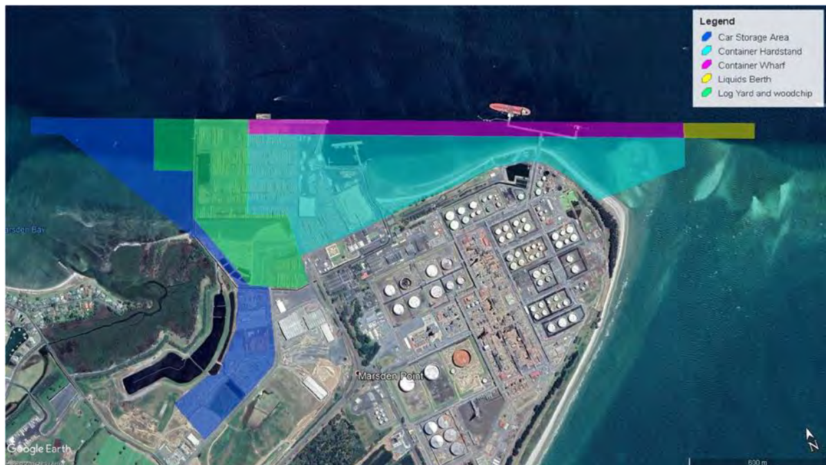
Figure 35: Concept layout for Northport expansion (forecast freight task, 2079)- Sapere, 2020
