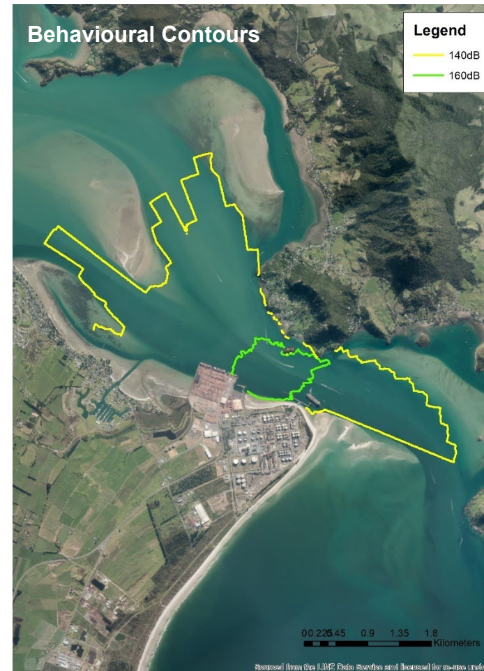
Figure 6. The predicted spatial ranges of the different functional hearing groups for the onset of temporary threshold shift (TTS; left) and the onset of behavioural responses (right) from percussive impact piling at the eastern edge of the wharf area. LF = Low Frequency group, MF = Mid-Frequency group, PW = Phocid Pinniped group in water and OW = Otariid Pinniped group in water. NOTE—These diagrams show sound contours from a pile source within the eastern reclamation area as this location was deemed the ‘worst-case scenario’ in terms of potential impact on visiting marine mammals (Pine 2022).
