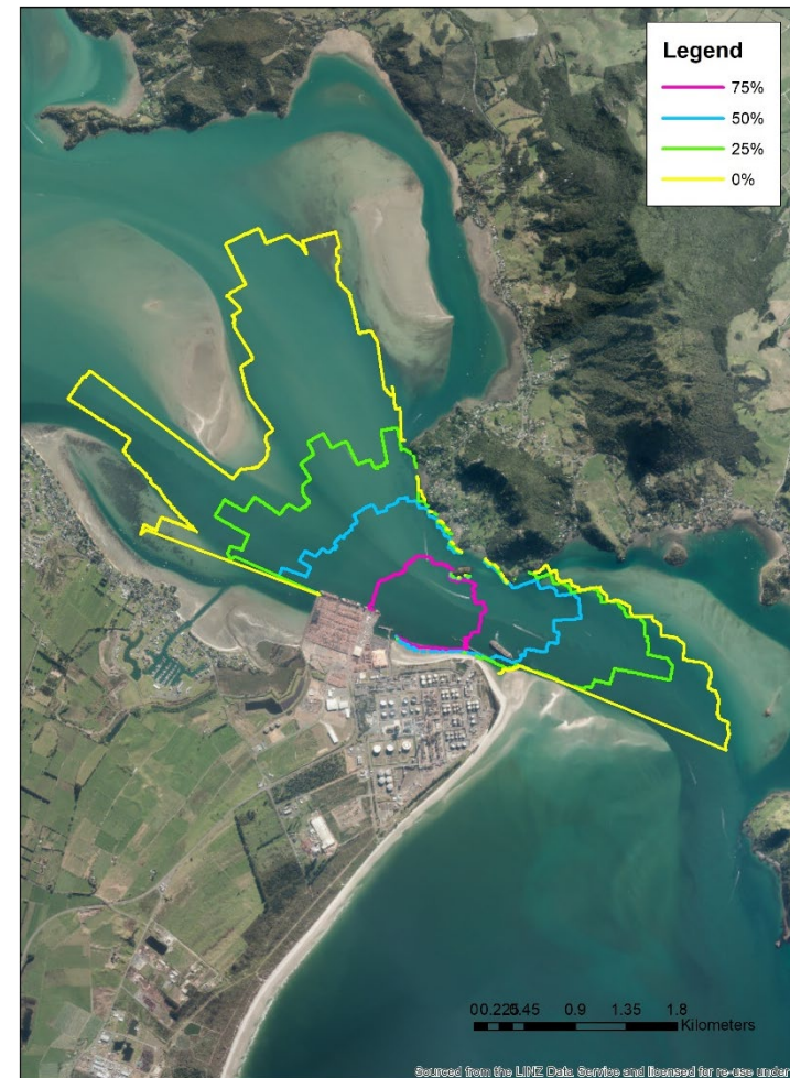
Figure A5.2 Distance contour plots of the predicted levels of reduced listening space risk (as a percent) from percussive impact piling for phocid animals in water (e.g. leopard seals swimming under water) on the left and otariid animals (e.g. fur seals swimming under water) on the right. For instance, the pink contour signifies the area around pile-driving activities where an animal's listening space has reduced to 75% of its unimpacted extent due to acoustic masking effects (Pine 2022).
