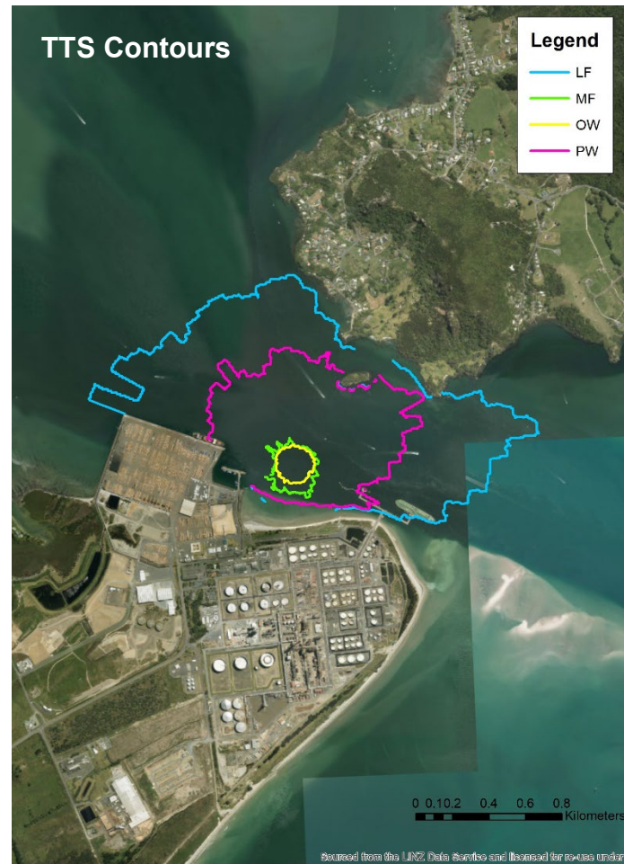
Figure 6. The predicted spatial ranges of the different functional hearing groups for the onset of temporary threshold shift (TTS; left) and the onset of behavioural responses (right) from percussive impact piling at the eastern edge of the wharf area. LF = Low Frequency group, MF = Mid-Frequency group, PW = Phocid Pinniped group in water and OW = Otariid Pinniped group in water. NOTE—These diagrams show sound contours from a pile source within the eastern reclamation area as this location was deemed the ‘worst-case scenario’ in terms of potential impact on visiting marine mammals (Pine 2022).
