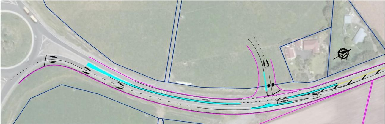
Figure 8: Downstream weave from seagull intersection to roundabout
