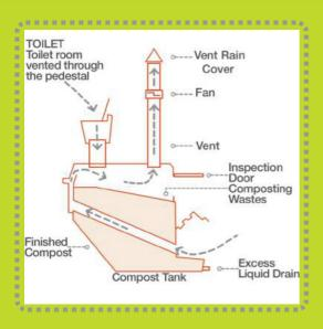
The Clivus Multrum™system is based on a "Continuous" composting process in one large chamber. As the organic material decomposes it will reduce in volume by up to 90%. The compost pile is therefore always 'shrinking in the middle' whilst new material is being added to the top, and finished compost is removed from the bottom of the pile as required.
